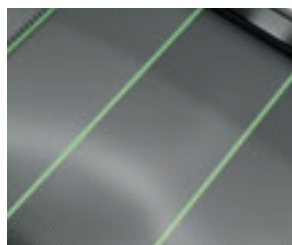
Pallet demarcation lighting
